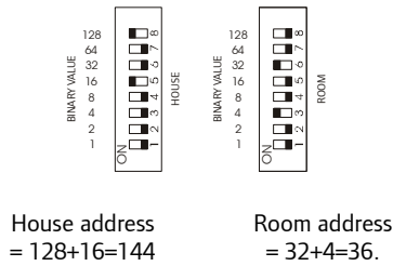
Fig 3. Addressing Switches
