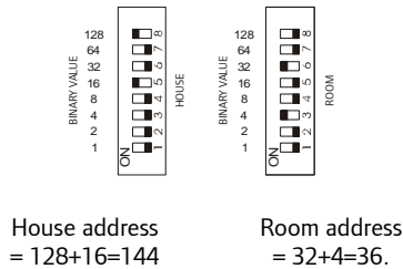
Fig 3. Addressing Switches
