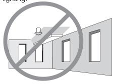
Move the Daylight Sensor to a location away from the lighting or lower it below the lighting fixture.
