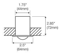
2" (50mm) diameter hole required for installation
