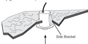
Do not place Daylight Sensor above indirect lighting.
