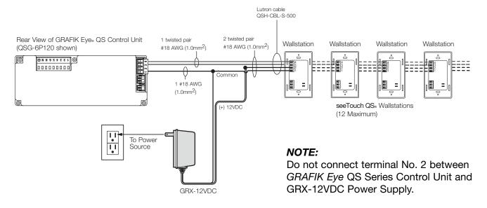
The +12 VDC wire from the power supply connects to QS link terminal 2 on all of the wallstations it is powering. This wire does not connect to terminal 2 on the *GRAFIK Eye* QS.
