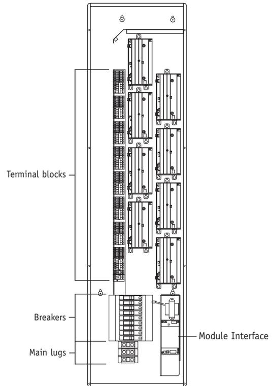
**Remote Power Panel with input breakers
